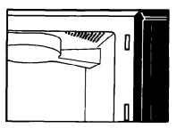
**NEVER** remove the mode mixer cover. The plastic cover protects the microwave mixer blade from soil or bending.
