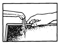
3. Soak grease filters in hot water and a mild detergent. Scrub and swish to remove embedded dirt and grease. Rinse well and shake to dry. Do not use ammonia or place in a dishwasher. The aluminum will darken.
